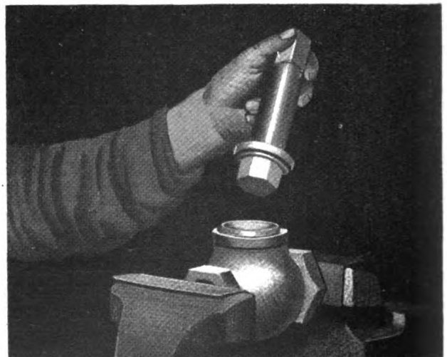
Figure 69. Steps in repairing globe valves.
